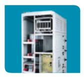
The MODIS ULTRA LV system is a fully type tested switchboard assembly compliant with the latest EN/IEC 61439-2 standards and is certified by ASTA. The system is available in 1250A, 1600A, 2500A and 3200A busbar ratings with certified shot circuit rating of 50kA for 3 sec. The system is also certified for temperature rise at an ambient operation of 50°C
